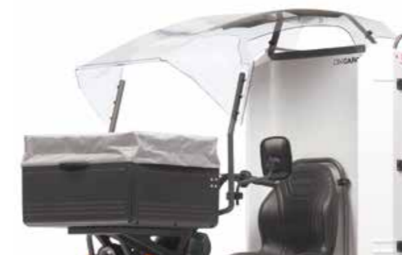
Roof (weather protection)
