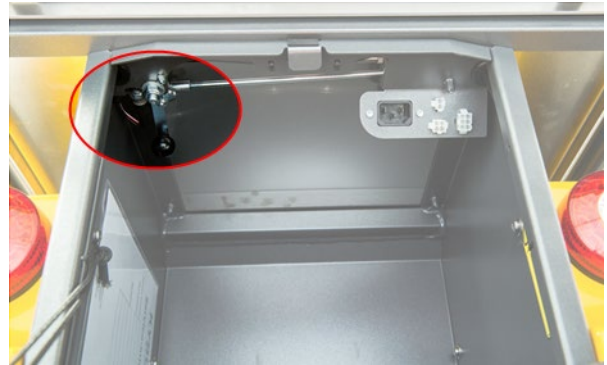
Position 2: Parking brake is activated and the vehicle is ready for use.
